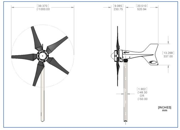
Rotational speed - 0-2000 rpm Swept area - 0.785m<sup>2</sup> Tip speed ratio - 6 Typical noise level - 6dB(A) above background Alternator type - Direct drive, axial flux, 8 pole permanent magnet generator Design - 3-phase AC with rectification Mounting - 48.3mm/50mm outer diameter pole
