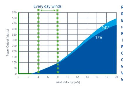
Rotor diameter - 1 metre Rotor Type - 5-Blade upwind Blade Material - Glass Reinforced, UV resistant Nylon Rated output - 105W at 8m/s (18mph, 15.5knots ) Peak output - 450W Cut-in speed - 3m/s (6.7mph, 6knots) Cut-out speed - None Weight - 8Kg Voltages - 12V, 24V, 48V DC, Grid-tie Warranty - 2 years
